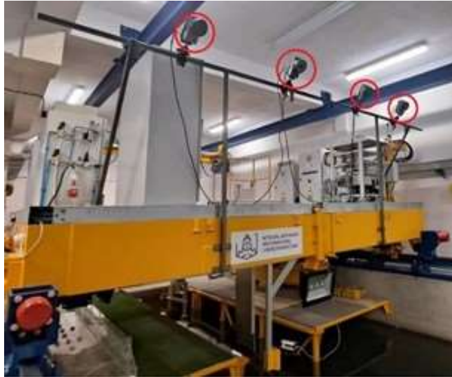
Figure 2.10 Gdańsk Tech Towing Tank with QualiSys cameras fitted on carriage
