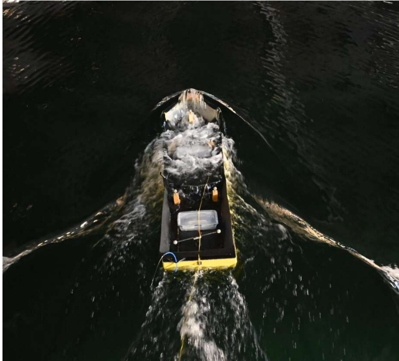
Figure 3.26 Water on deck as a result of wave blocking in case B38
