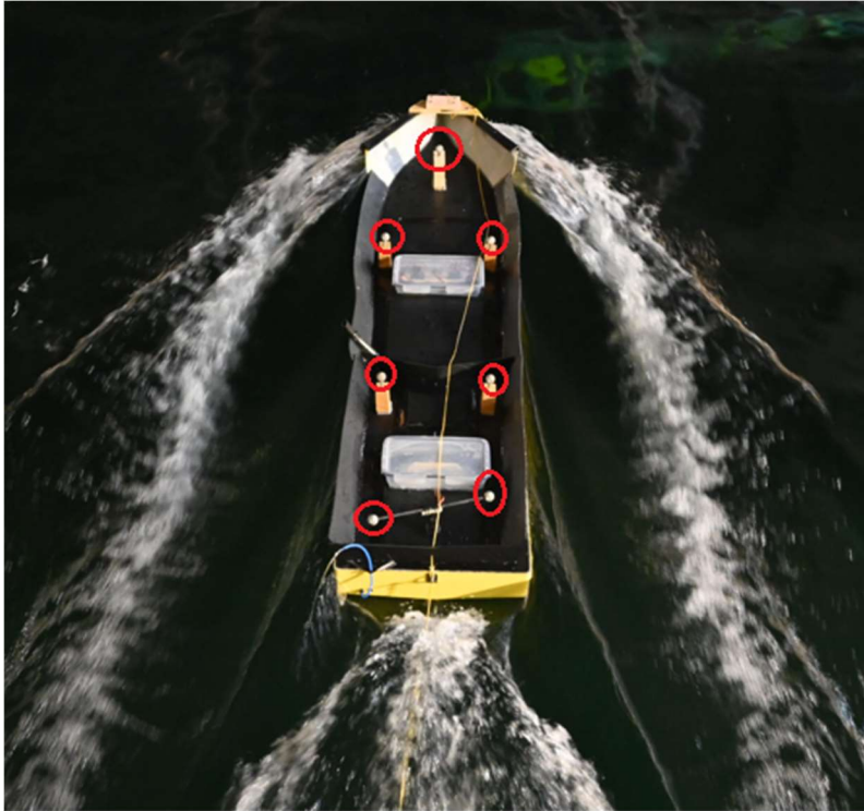
Figure 2.4 1/14 scale model with the passive markers marked with red circles
